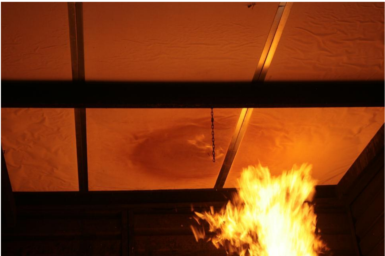
Figure 4.1.8: Sporadic ignition and widening discolouration area above fire source area
