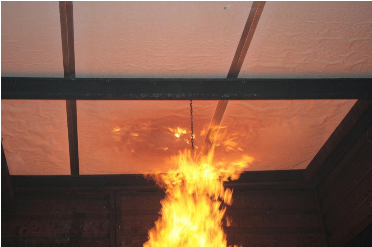
Figure 4.1.7: Note sporadic ignition above fire source area
