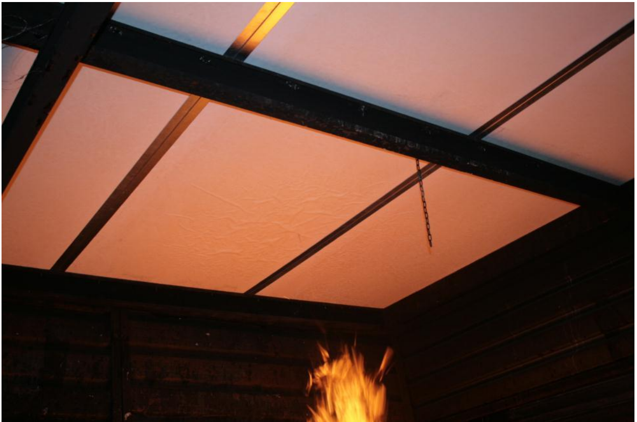
Figure 4.1.4: Note the wrinkling of the facing material above the fire source.
