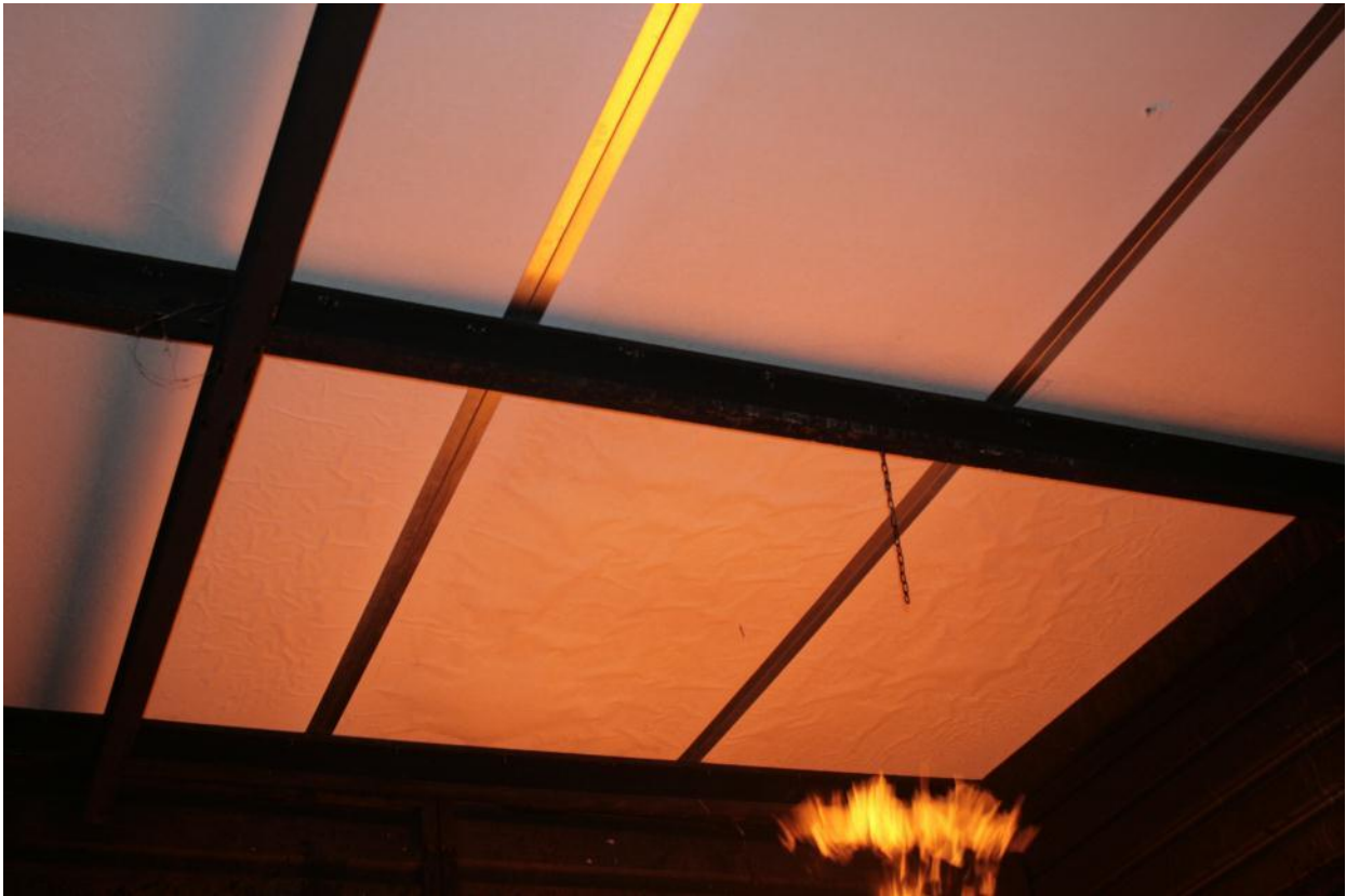
Figure 4.1.5: Note delamination of facing material above fire source.
